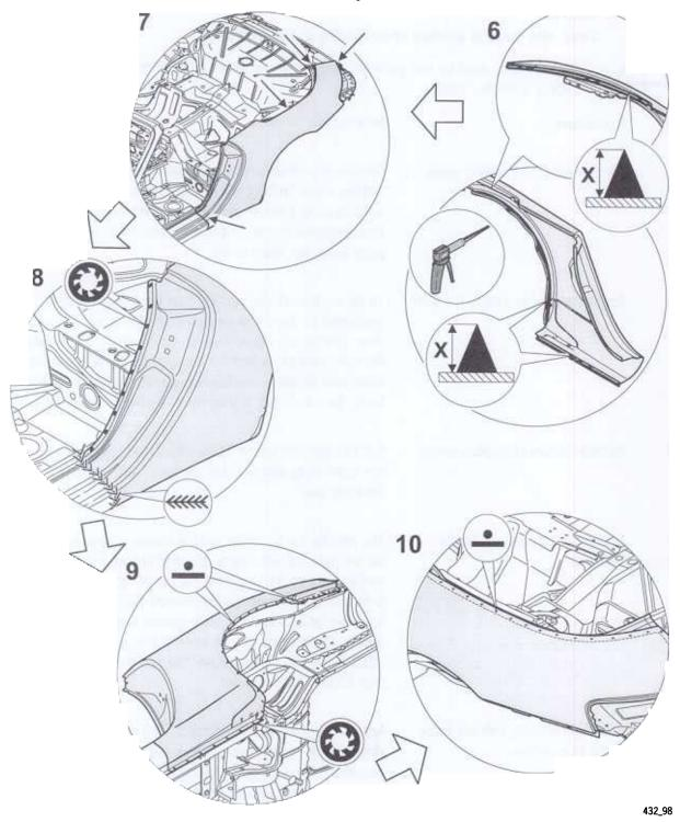
Inserting the side section - Cabriolet into the body
