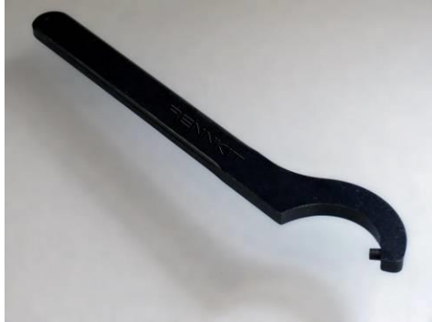
Figure 2b: Renntool™ Pin Wrench (available at www.renntool.com/purchase )
