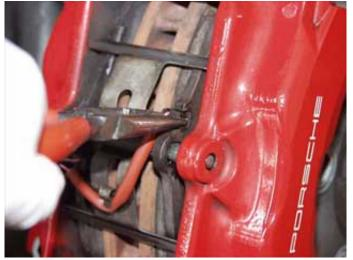
Step 3: Remove the "Pad Retaining Spring Retaining Pin Retaining Clip" ...
