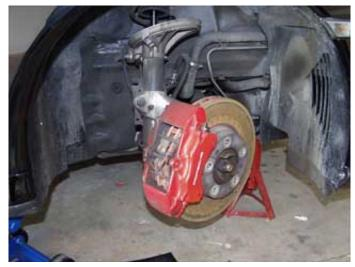
**Step 2: Remove the Low-Pad-Warning Sensors**
