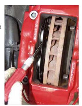
In either case, note that the inner diameter of the upper piston is bigger than the lower one, so there are two different size antirattle clips. You might not notice this until you try to reinstall them. So I thought I'd point it out now.
