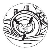
4. Tighten fastening screws on servo pump Tighten the fastening screws of the servo pump drive wheel.
