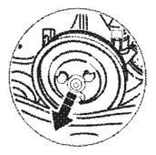
4. Remove servo pump wheel
