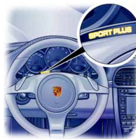
SPORT/SPORT PLUS display on the PDK steering wheel with shift buttons
