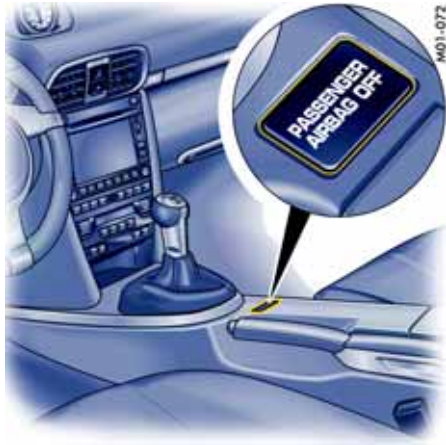
PASSENGER AIRBAG OFF indicator lamp
