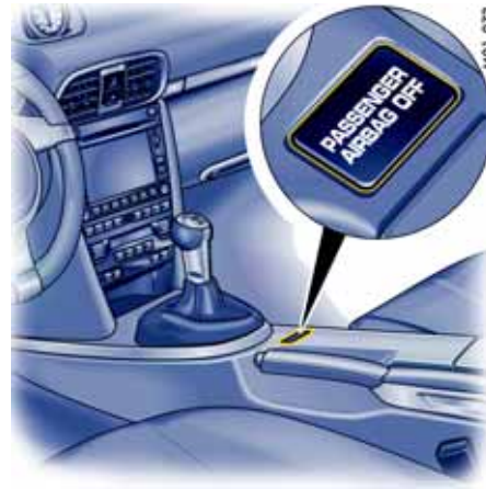
PASSENGER AIRBAG OFF indicator lamp
