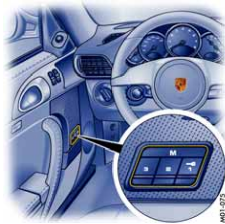
M - Memory button 1 - Key button 2, 3 - Person buttons
