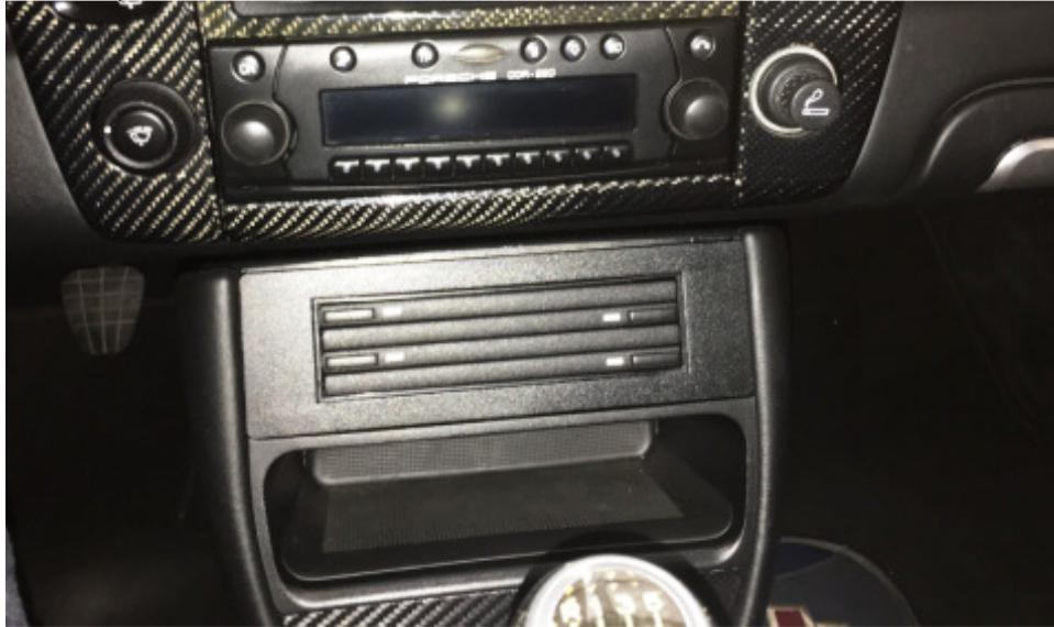
On these set of pics the only note I would say during radio removal is that a firm grip is necessary. I found that using my ring fingers on both hands and creating a fist is what allowed me to get enough leverage to pull out the radio as my index and middle fingers were too big and would cut easily. (*Note; the instructions suggest putting two screw drivers through the rings*)
