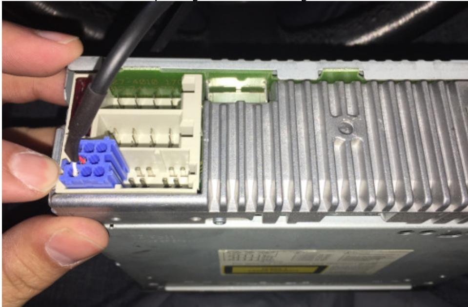
More pictures of where to guide the wires. Once I got the 12ga. wire down and into the bottom cubby area then I taped the aux jack to the 12ga wire and pulled it through to the bottom as the blue connector on the end of it is tough to fish upwards. After that was fished through, I then taped the BT converter harness/inline fuse to the 12ga wire from bottom cubby area and pulled it UP through. I found it to be a lot easier this way.
